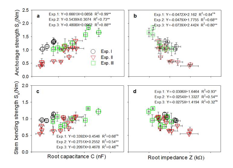
EC and impedance displayed consistent relationships with anchorage strength and stem bending strength in all three field expts
