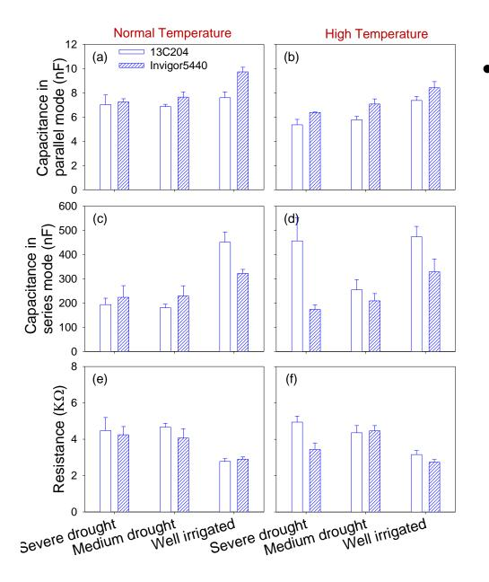
Clearly, capacitance in parallel mode detected genotypic differences in response to stress
