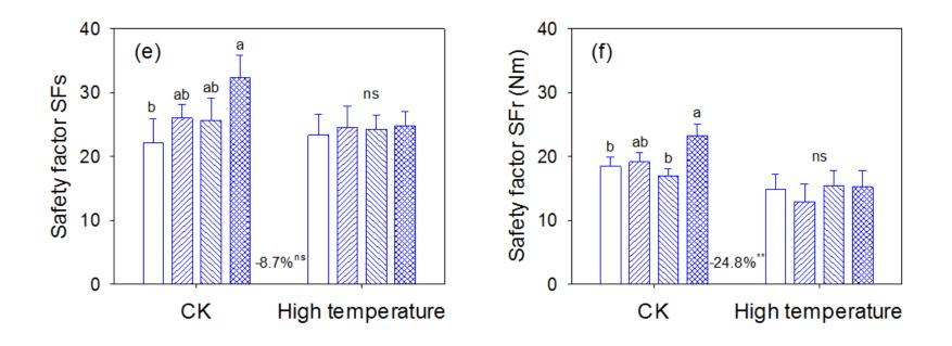
High temperature significantly reduced root safety factor by 24.8 %; but only reduced stem safety factor slightly
